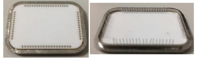
Figure 4: Images of the Hub electronics 64-pin Feedthrough Plate. External side (left), internal side (right)
