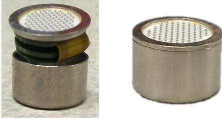
Figure 13: Images of the satellite electronics system. Exploded view of the folded board mounted to the feedthrough substrate (left), Enclosed system (right).
