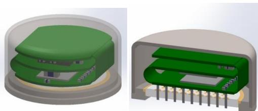
FIGURE 4: FULL AND CROSS SECTION ILLUSTRATIONS OF THE SATELLITE SYSTEM.
