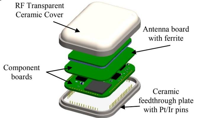
FIGURE 7: EXPLODED VIEW OF THE HUB SYSTEM ELECTRONICS PACKAGE.
