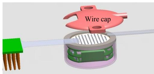
FIGURE 5: SATELLITE SYSTEM ILLUSTRATING THE FEEDTHROUGH PLATE RECESS FOR WIRE ATTACHEMENT AND THE WIRE CAP USED FOR PROTECTION OF THE WIRES AND SECURING THE SYSTEM TO THE SKULL.
