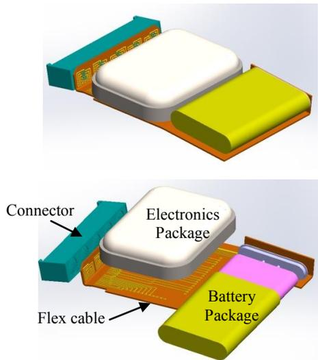
FIGURE 6: ILLUSTRATION OF THE HUB SYSTEM OVERVIEW (TOP) AND EXPLODED VIEW (BOTTOM).
