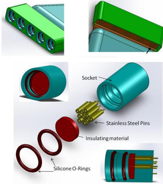
FIGURE 8: ILLUSTRATION OF THE CONNECTOR HOUSING AND SOCKET FOR LINKING THE INDIVIDUAL SATELLITES UP TO THE CENTRAL HUB SYSTEM.
