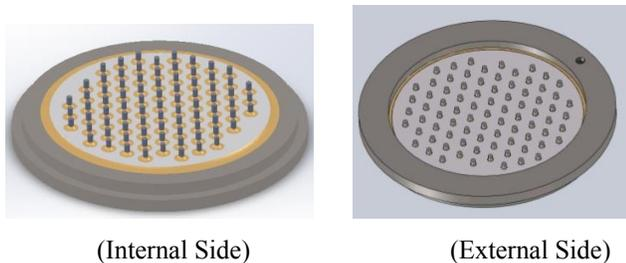
FIGURE 3: ILLUSTRATION OF THE INTERNAL AND EXTERNAL SIDE OF THE SATELLITE CERAMIC FEEDTHROUGH PLATE.
