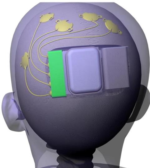
FIGURE 1: ILLUSTRATION OF THE PACKAGING ARCHITECTURE OF INDIVIDUAL SATELLITES CONNECTED TO A MAIN HUB SYSTEM.
