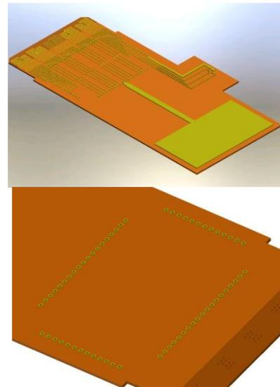
FIGURE 9: ILLUSTRATION THE TOP AND BOTTOM SIDE OF THE FLEX CABLE.
