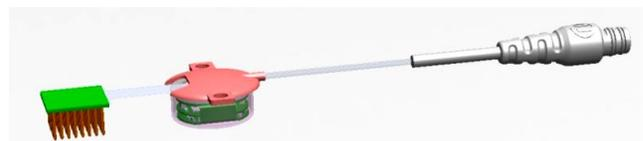
FIGURE 2: ILLUSTRATION OF THE SATELLITE SYSTEM CONNECTED TO A MICROELECTRODE ARRAY AND A HUB SYSTEM CABLE.
